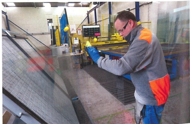
Right: Hegla Optimax cutting table with the loader in the background (reverse view above).
