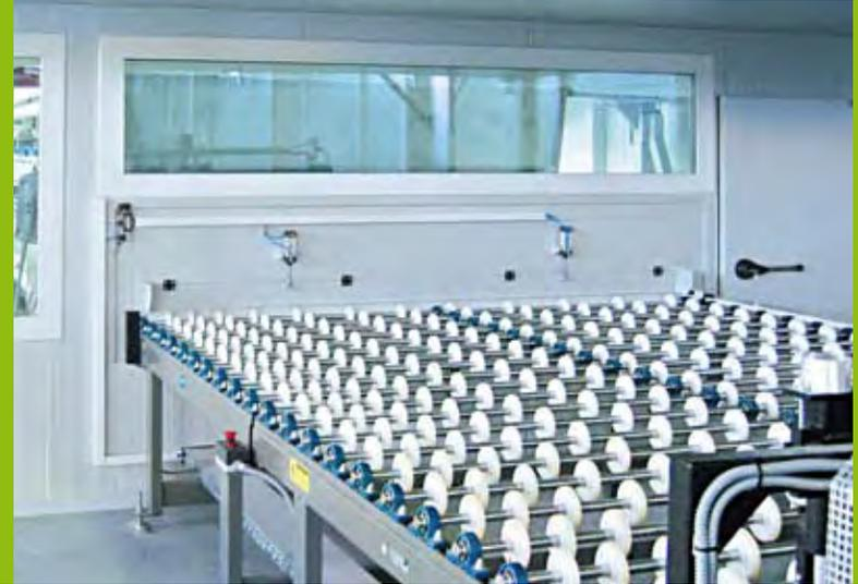
If there is no glass to be washed in the washing machine during the production of laminated glass and insulating glass, the ventilation flaps of the blower close. The result: 25% energy saving.
