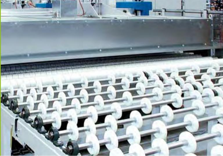
In photovoltaic module production, we replace the vacuum laminators by a pre-nip with press rollers.
