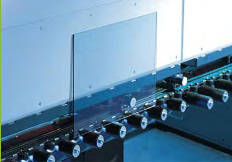
What is temporarily not in use does not have to be driven. Using shared drives in the production of laminated glass and insulating glass, we ensure that only those conveyor units are running which carry glass at the specific moment. All the others are motionless.
