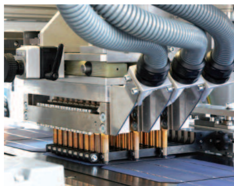
Soft touch soldering system
