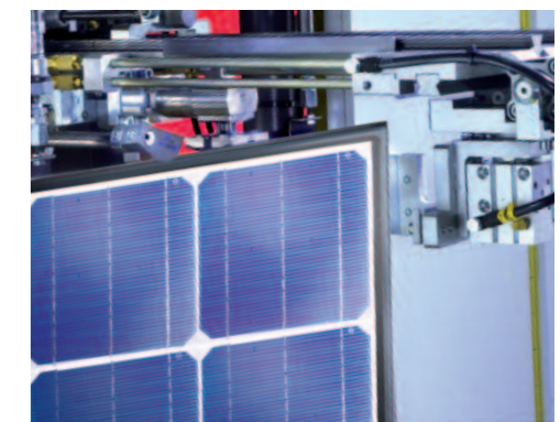
Automatic, homogeneous sealing of TPedge module
