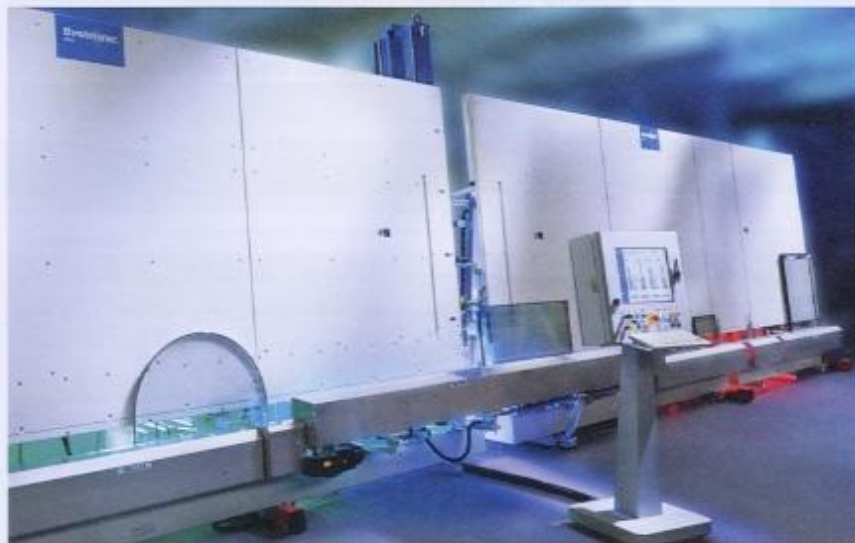
The speed'sealer, a high-speed sealing robot for insulating glass unit production
